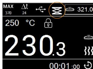
In case of interruption of the data connection between the lab jack and magnetic stirrer, the following warning appears on the display of the magnetic stirrer [73: Lab jack has no connection] and the [Lab jack connected] symbol goes out.
